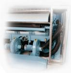
vacuum fans for optimum drying capacity while minimizing back pressure. The very large 4" outlet bore in the left side roll shafts, which are supported by very large 6.3"-diameter roller bearings, maximizes this drying capacity.
