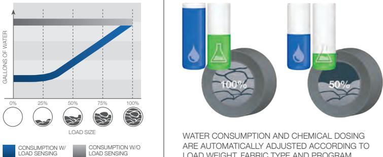
The graph plots 'GALLONS OF WATER' on the y-axis against 'LOAD SIZE' on the x-axis (0%, 25%, 50%, 75%, 100%). A blue line shows that water consumption increases proportionally with load size. Below the graph, two circular diagrams illustrate '100%' and '50%' load levels with corresponding water and detergent dispensing.
